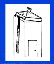
Roof ventilation is critical for search, rescue and extinguishment of the fire. Relieves the upper portions of the building of heat, smoke and gases, limiting horizontal spread.
