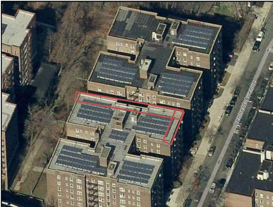
Example of required clear paths to comply with the NYC Fire Code. The red indicates clear paths on one section of the building but note that clear paths are required on each part of the “H”-shaped roof. Although the NYS Fire Code sets minimum requirements for building access, specific requirements vary by jurisdiction.
